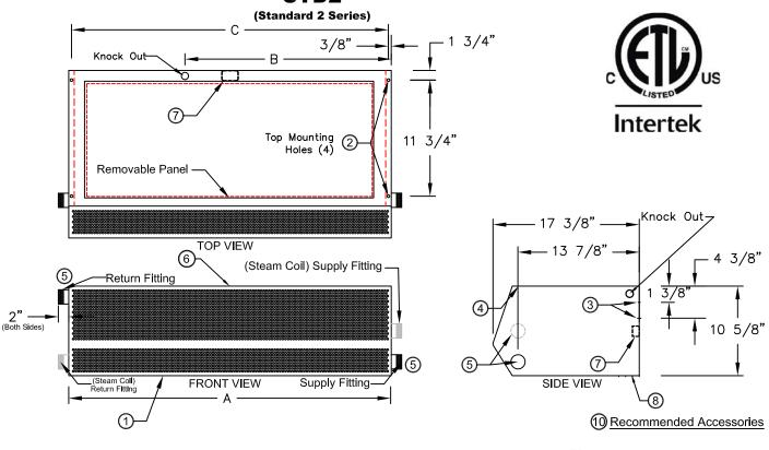
Use corresponding letters in "Coil Data" then "Electrical Data" columns to complete the model numbers.
